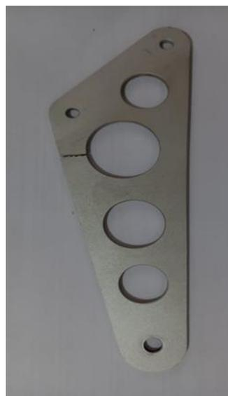
**FIG 1 ( DISEÑO ORIGINALCON FRACTURA)**
